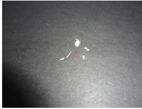
Above: Items removed from north beamtube bellows
