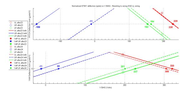
Interestingly the only difference between the measurement of the plots above is the ESD LL quadrant cabling going through the ESD LP filter box instead of BIAS and they are 1 day apart. We see how most of quadrants do not have a big change in charge with the exception of the quadrant with opposite sign charge which has now charged with the same sign as the rest of quadrants.
