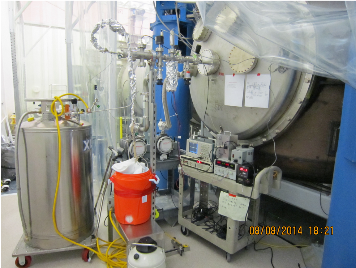
Figure 1 The ionizer attached to the ETMY chamber as configured for the second test. The instrument is described in T1100332 and G1100364. The new elements not part of the initial test on the MIT LASTI facility are the additional liquid nitrogen trap in the fill line and the gas reheating section between the trap and the entry into the ionizer. The additional trapping was to avoid oil and water frozen dust that could be at the bottom of the storage dewar from entering the test mass chamber. Prior measurement had determined that both the hydrocarbon and dust emission at the ionizer output was small enough to avoid contamination of the optics. The single post support bolted to the ground was effective.
