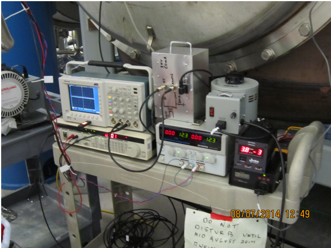
Figure 3 The instrumentation for the ionizer. The oscilloscope displays the 60Hz current between the needles and the vacuum shell (ground) as well as the currents of positive and negative ions that make it into the flow after the apertures. The sampled current is about 1/100 of the current in the flow. The variac controls the voltage on the needles.
