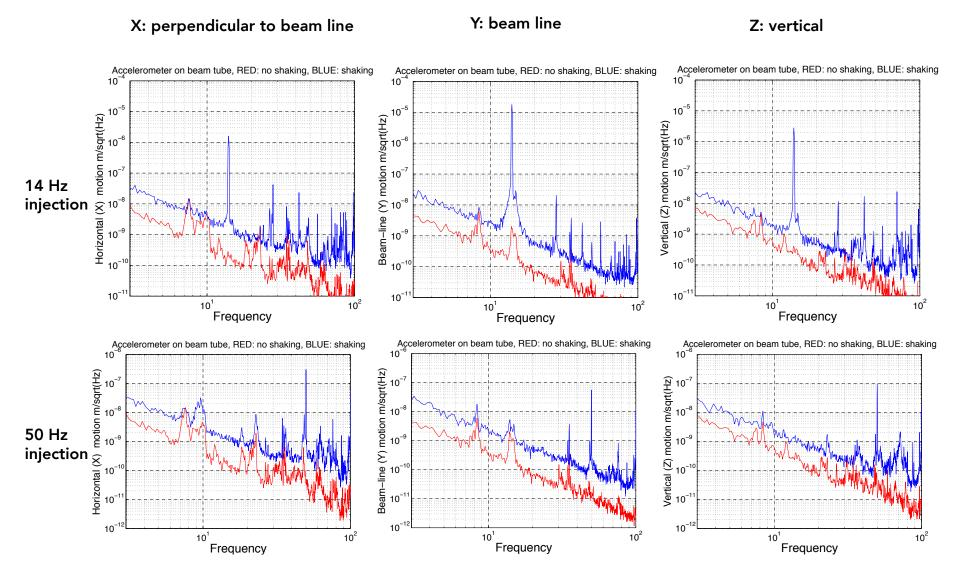
Note: noise floor is higher for injections because accelerometer gain had to be reduced by 10
