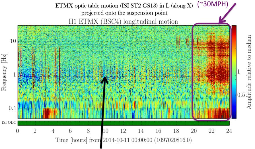
Most of the day, Oct 11, high microseism, low wind (~5MPH)
