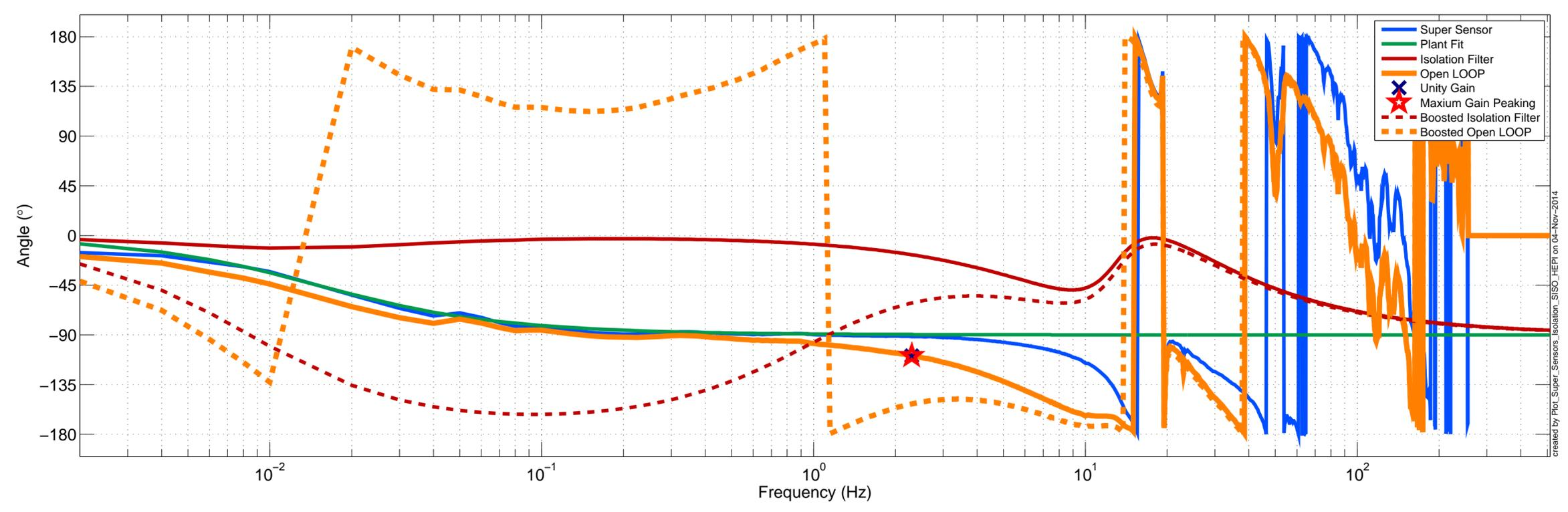
2013\_09\_04--H1\_HPI\_HAM2--Super Sensor - VP Control Lvl 1 The maximum gain peaking 1.18 is obtained at 47.5 Hz.
