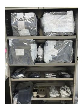
One storage container is on the shelves just inside the air shower on the second shelf to the left. The spare PD array cover and spare strain relief assembly are on the right.
