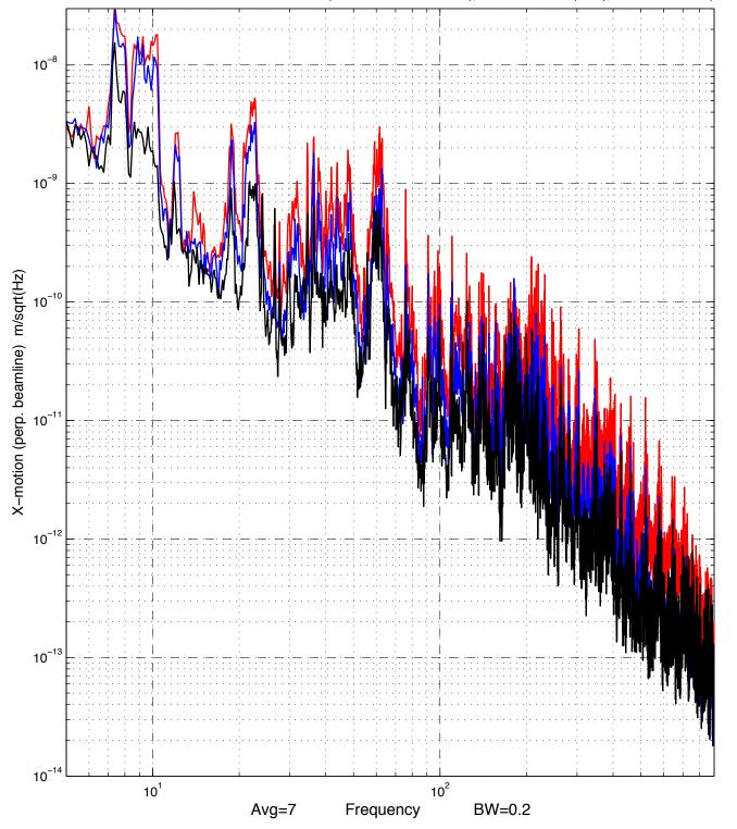
Beam tube at baffle #96 near MY. RED: 24 MPH (exceeded 12% of hours), BLUE: 18 MPH (25%), BLACK: 9 MPH (65%)
