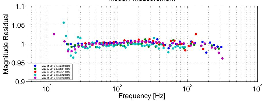
Latest DCC Pole Freq: 303 [Hz], ESD Pole: 2200 [Hz]
