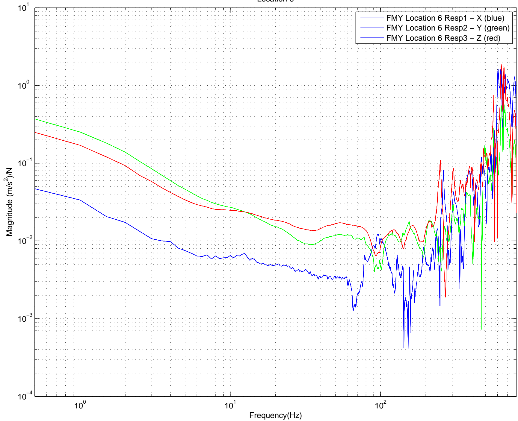
FMY Tap Test – M0 & R0 Damping ON – ISI Floating Location 6
