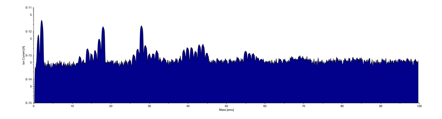
~1138 hrs local -> Y-end open to BT, with 3.5x10-8 torr\*L/sec N2 leak on and pumped by NEG
