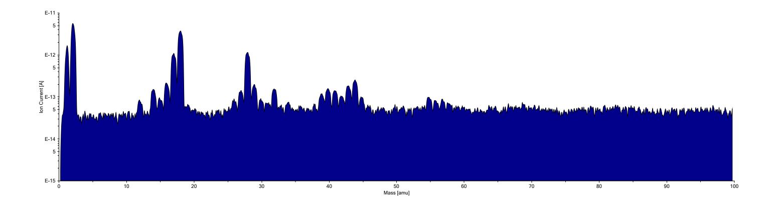
~1428 hrs. local -> Y-end open to BT, pumped by NEG and with 3.5x10-8 torr\*L/sec N2 leak on
