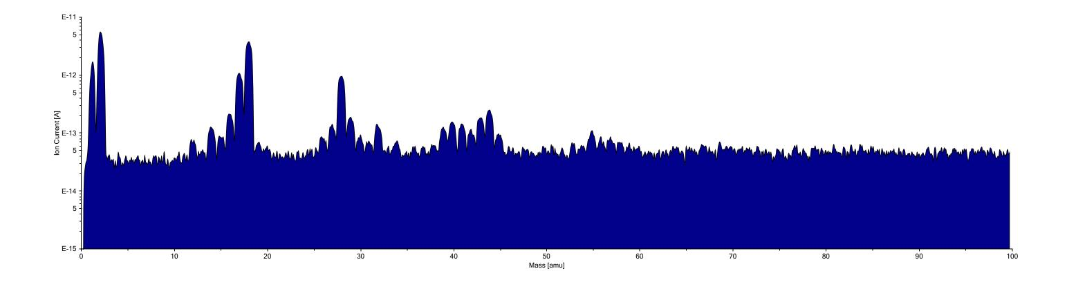
~1438 hrs. local -> Y-end open to BT, pumped by NEG and with 3.5x10-8 torr\*L/sec N2 leak off
