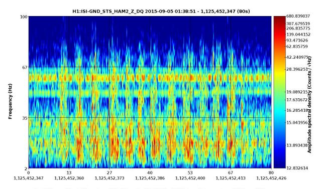
$Fs = 512 Hz, \ sec/fft = 0.50, \ overlap = 0.90, \ fft \ length = 256, \ \#-FFT = 1566/1, \ bw = 2, \ in \ samples = 41 K, \ low = 0.20 Hz, \$
