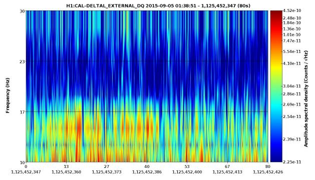
$Fs = 16,384 Hz, \ sec/fft = 0.50, \ overlap = 0.90, \ fft \ length = 8,192, \ \#-FFT = 1589/1, \ bw = 2, \ in \ samples = 1,311 K, \ low = 0.20 Hz = 1,000 Hz = 1,00$
