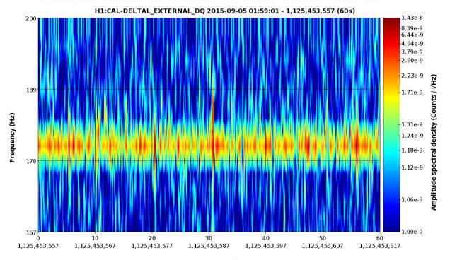
Fs = 16,384 Hz, sec/fft = 0.50, overlap = 0.90, fft length = 8,192, #-FFT = 1189/1, bw = 2, in samples = 983 K, low = 0.20 Hz = 100 Hz =
