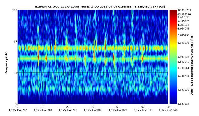
Fs=2,048Hz, sec/fft=0.50, overlap=0.90,  $fft\ length=1,024$ , #-FFT=1581/1, bw=2,  $in\ samples=164K$ , low=0.20
