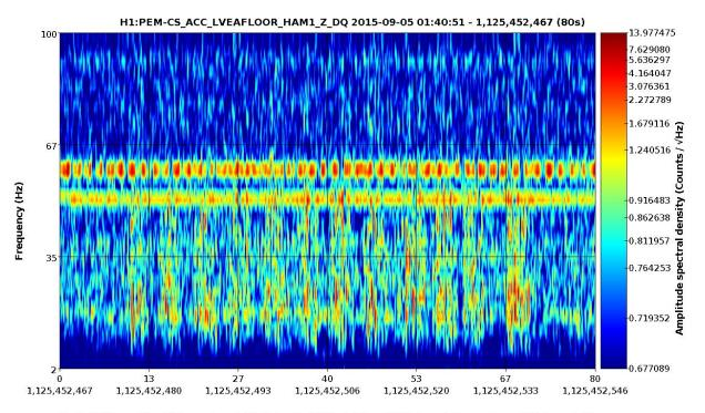
$Fs = 2,048 Hz, \ sec/fft = 0.50, \ overlap = 0.90, \ fft \ length = 1,024, \ \#-FFT = 1581/1, \ bw = 2, \ in \ samples = 164 K, \ low = 0.20 Hz = 1.00 Hz =$
