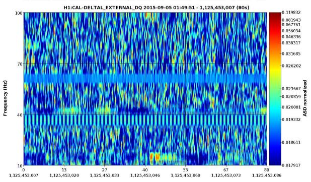
$Fs = 16,384 Hz, \ sec/fft = 0.50, \ overlap = 0.90, \ fft \ length = 8,192, \ \#-FFT = 1589/1, \ bw = 2, \ in \ samples = 1,311 K, \ low = 0.20 B, \ low = 0.$
