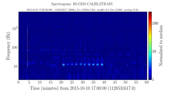
The only structure visible in the spectrogram is a large glitch at ~4 mins and unrelated PEM tamper injections above 10 Hz from 20 - 40 mins. Nothing that indicates coupling from the RF injection.
