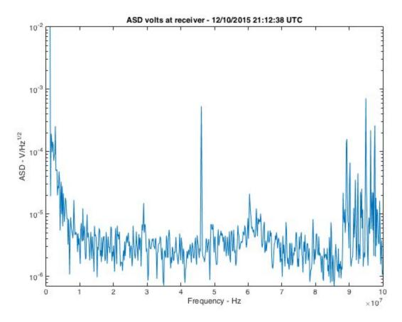
While the wideband scanner has good sensitivity and is able to cover a large range of over 100 MHz, it does suffer from a lack of time and frequency resolution, for this sweep it had a frequency resolution of  $\sim$ 100 kHz and took a spectrum measurement about once a second.
