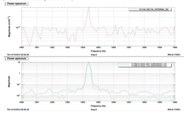
Based on our known coupling in the 45 MHz band and the fact that the sweep was in the band for only 200 ms it is not expected to have been visible in darm. If our signal had remained in the band for ~few seconds we would expect to see it in darm when it passed through 45MHz, however to scan the whole band at that speed would have taken many hours.
