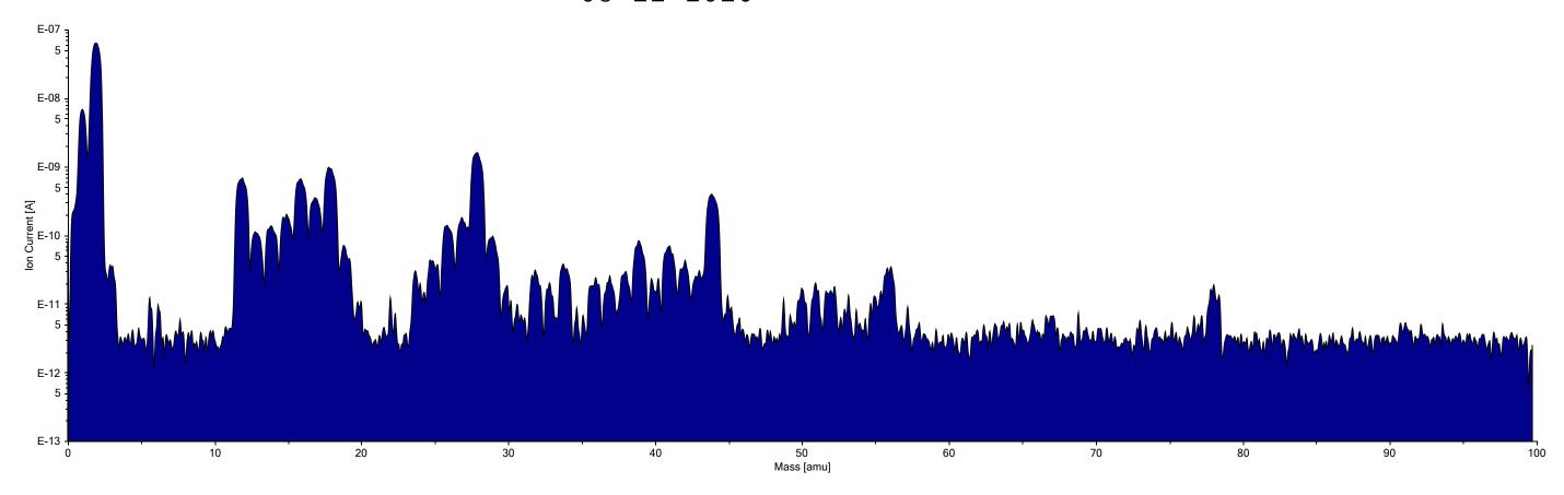
LHO Y-end RGA following bake out, pumped by locally mounted turbo (est. net pump speed  $< 10 \ l/s$ ), SEM mode 1500 volts
