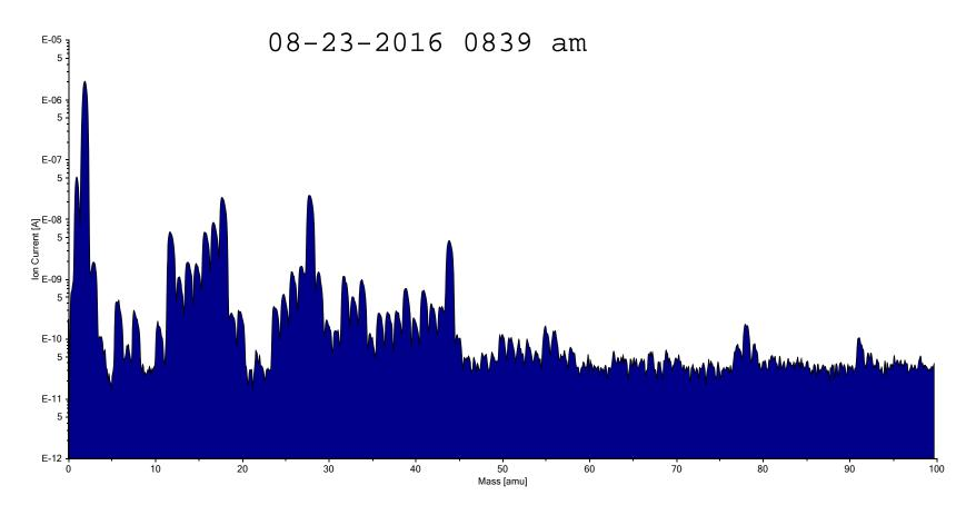
Vertex RGA pumped by locally mounted turbo ( $\sim 10 \text{ L/s}$ ), isolated from Vertex Vacuum Volume and with calibration gases isolated - SEM 1500 volts
