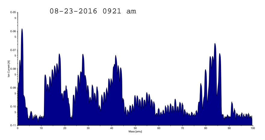
Vertex RGA pumped by locally mounted turbo (~10 L/s), isolated from Vertex Vacuum volume with 4 x 10-8 torr\*L/sec krypton leak open SEM 1500 volts
