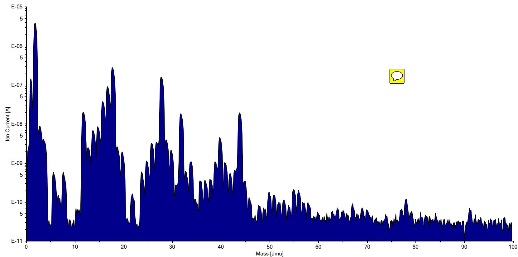
Vertex Vacuum Volume, locally mounted turbo and calibration gases isolated, conductance from RGA ~100 L/s, SEM 1500 volts
