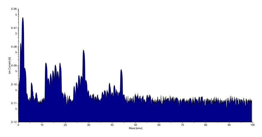
LHO Vertex RGA while isolated from the Corner Station and while pumped by the locally mounted turbo (with an air leak confirmed at the turbo vent valve). SEM = 1500 volts.
