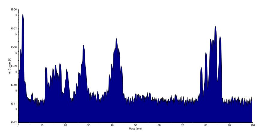
LHO Vertex RGA while isolated from the Corner Station, pumped by the locally mounted turbo (with an air leak confirmed at the vent valve) and with the locally mounted  $3.3 \times 10-8$  torr\*L/sec Krypton leak open. SEM = 1500 volts.
