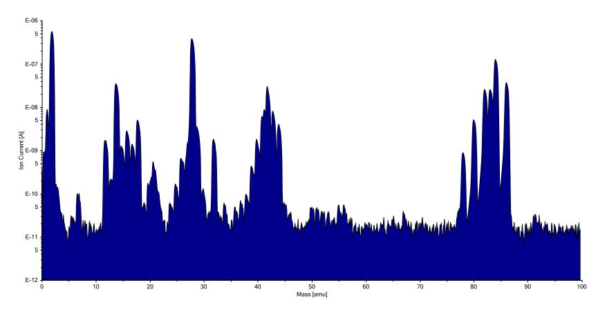
LHO Vertex RGA while isolated from the Corner Station, pumped by locally mounted turbo (with an air leak confirmed at the vent valve) and with the 3.3 x 10-8 torr\*L/sec Krypton and 3.3 x 10-8 torr\*L/sec N2 leaks open. SEM = 1500 volts.
