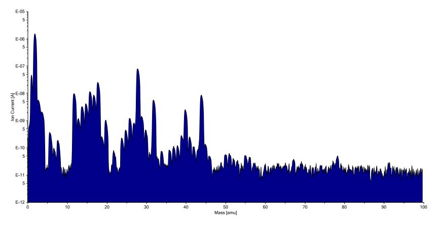
LHO Corner Station (while open to the arms) as seen by the Vertex RGA when the local turbo and calibration gases are isolated. SEM = 1500 volts
