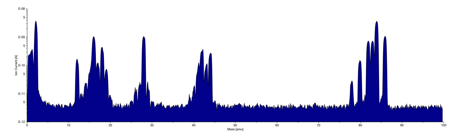
X-end RGA, isolated from X-end volume, pumped by locally mounted turbo ( $\sim 10~l/s~net$ ), Kr calibration gas open (5 x 10-8 torr\*l/sec), SEM = 1500 volts and with factory default ionizer settings
