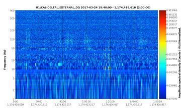
Fs=16,384Hz, sec/fft = 1.00, overlap = 0.50, fft length=16,384, #-FFT = 14399, bw = 1, in samples = 117,965K, low = 0.20
