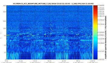
Fs=16,384Hz, sec/fft = 1.00, overlap = 0.90, fft length=16,384, #-FFT = 41976, bw = 1, in samples = 68,813K, low = 0.20
