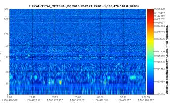
Fs = 16,384 Hz, sec/fft = 1.00, overlap = 0.90, fft length = 16,384, #-FFT = 41976, bw = 1, in samples = 68,813 K, low = 0.20 Hz, low = 10.00 Hz, low = 10.0
