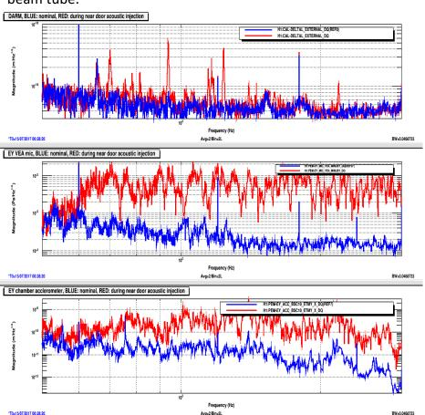
Likely bird pecks from Hveto, the sound from the peck is not loud enough (second row) to account for DARM (top row), but the chamber accelerometer signal is, so the direct vibrational coupling through the pipe to the vacuum envelope is the likely coupling route.
