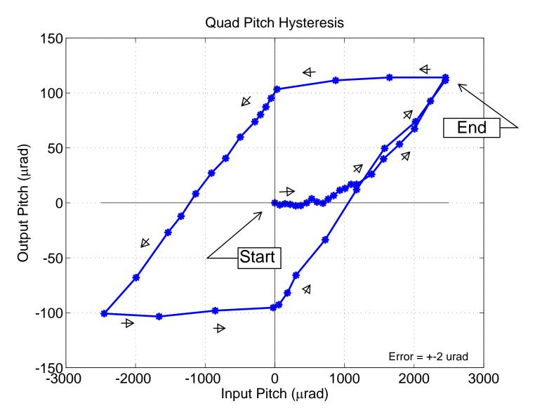
This plot shows the hysteresis as seen on the test mass of the reaction chain. The x axis is the input pitch, meaning the pitch angle the test mass acquired from an input torque at the top mass. The y axis is the angle the test mass came back to after the input torque was removed. The arrows show the path taken during the measurements. At maximum input the offset is 4.7%.
