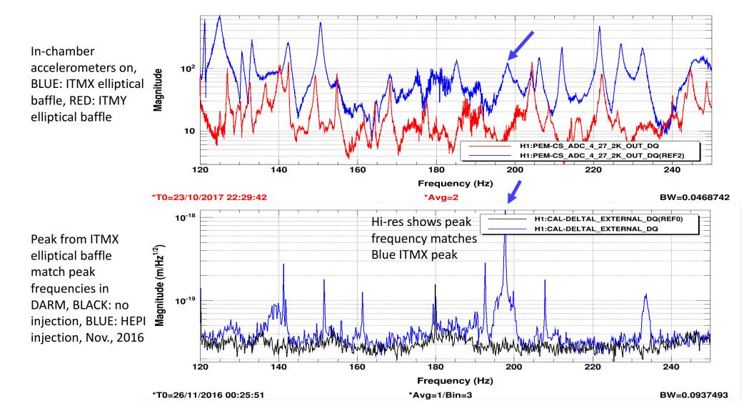
In-chamber accelerometers on, BLUE: ITMX elliptical baffle, RED: ITMY elliptical baffle
