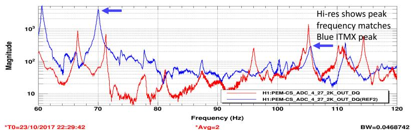
Peaks from ITMX elliptical baffle have been in DARM for a long time, BLUE: no injection, RED: shaker injection, Jun., 2016
