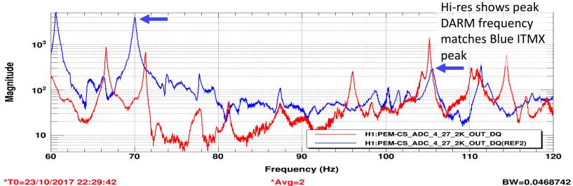
Peaks from ITMX elliptical baffle match peak frequencies in DARM, BLUE: no injection, RED: HEPI injection, Aug., 2017
