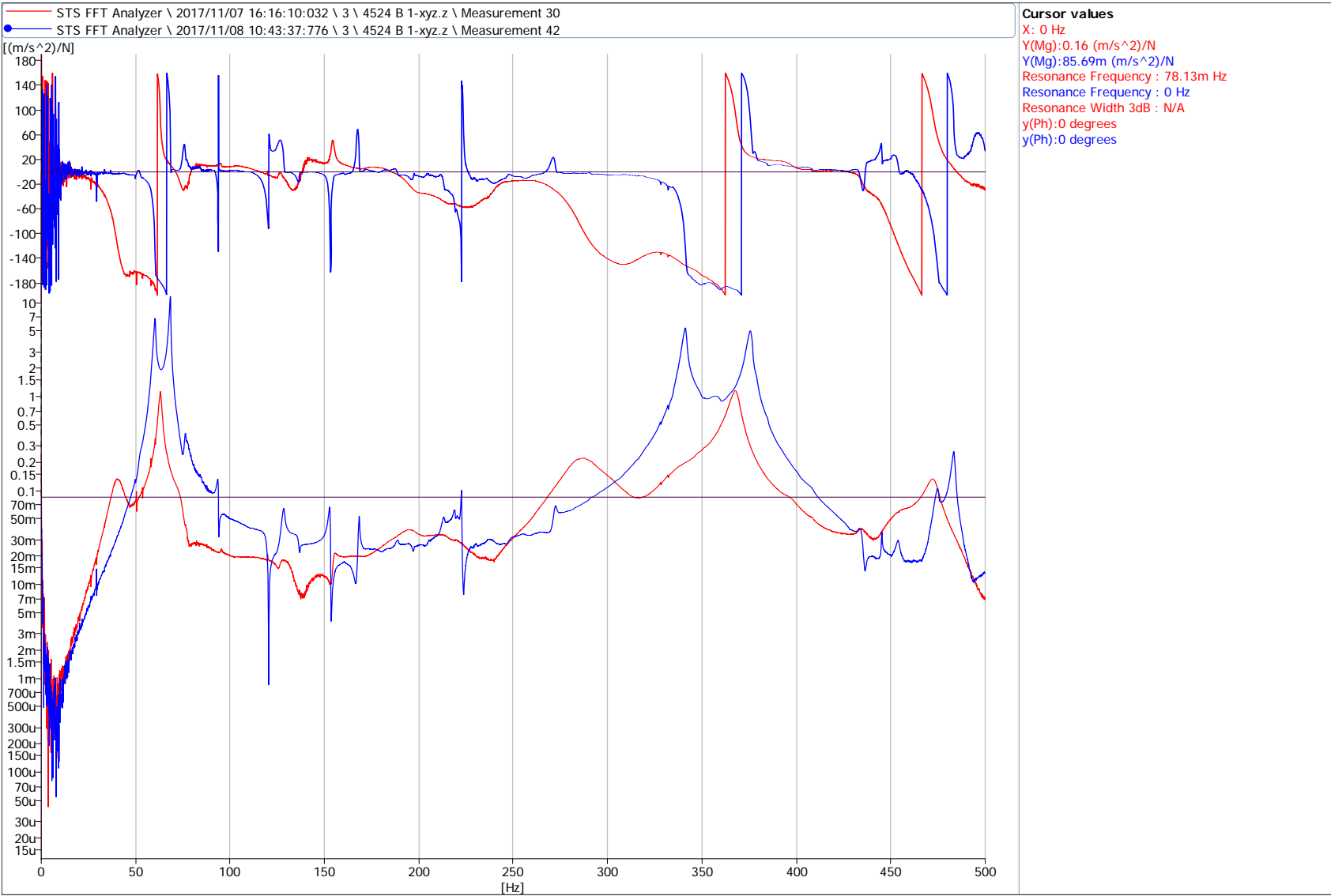
Figure 8. Damped versus undamped upper baffle, exciting directly on the baffle in longitudinal direction. Measurement 42 is undamped with stainless steel washers used as spacers in place of viton O-rings. Measurement 30 is damped with viton O-rings and mounting bolts turned 1/2 turn past hand tight.
