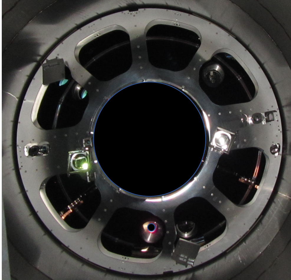
Figure 3. View from ETMY beam spot, before and after stray light upgrade, with optical lever beam and reflections from gate valve (at center), blacked out
