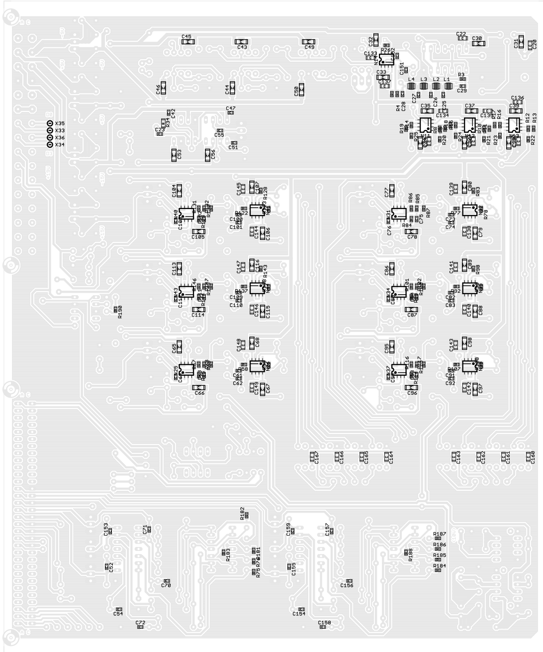
Figure 15: Board bottom view showing placeplan with component names
