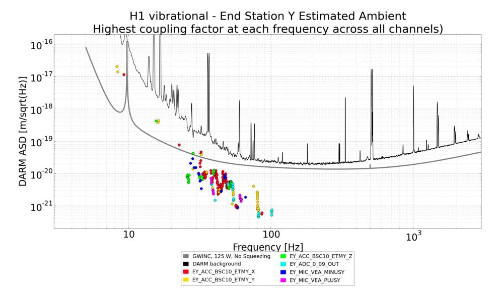
Ambient estimates are made by multiplying coupling factors by injection-free sensor levels. CIRCLES indicate estimates from measured coupling factors, i.e. where the injection signal was seen in the sensor and in DARM. TRIANGLES represent upper limit coupling factors, i.e. where a signal was not seen in DARM. For some channels, at certain frequencies the ambient estimates are upper limits because the ambient level is below the sensor noise floor.
