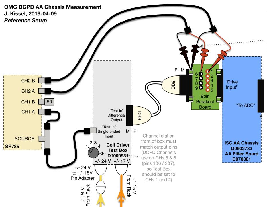
Shields of Differential Signal on BNC Returning to SR785 MUST be connected to the same ground as the shield on your "Test In" from the SRC
