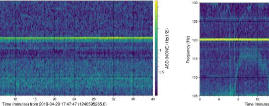
Spectrogram: H1:PEM-CS\_ACC\_ISCT6\_SQZLASER\_X\_DQ,raw fftlength=4.0, overlap=0.9
