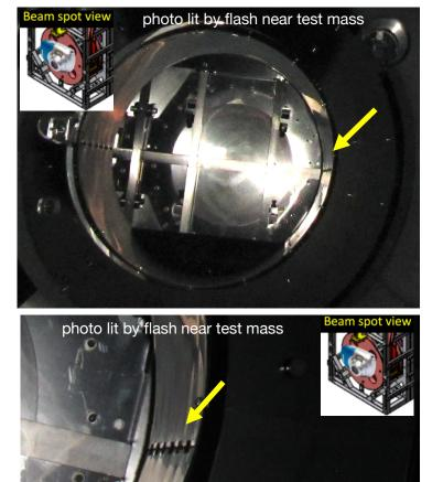
Can we extend the P-cal baffle to cover the barrel without clipping problems? We should at least plan to damp the barrel better.
