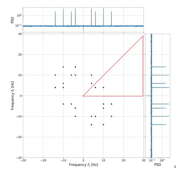
Note that if the bicoherence is high at a point (f1,f2), that means that the noise in DARM at f1+f2 is correlated with the "product" of noise at f1 and at f2
