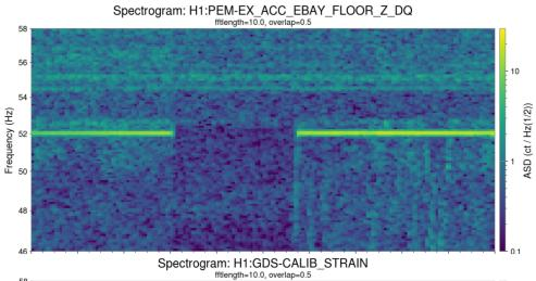
DARM showing 52 Hz peak disappears when pump off
