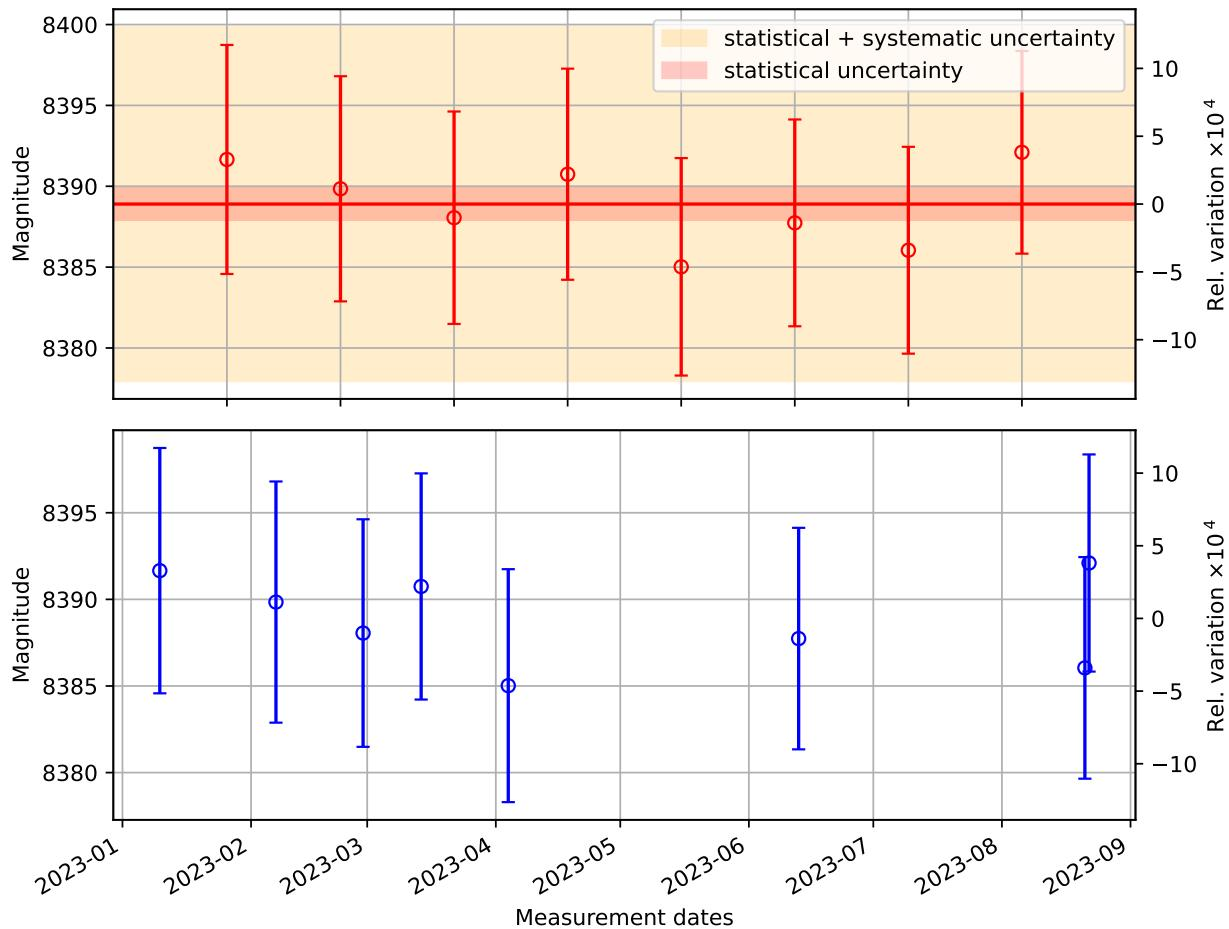
Summary of TxPD calibration corrected for optical efficiency (ct/W)
