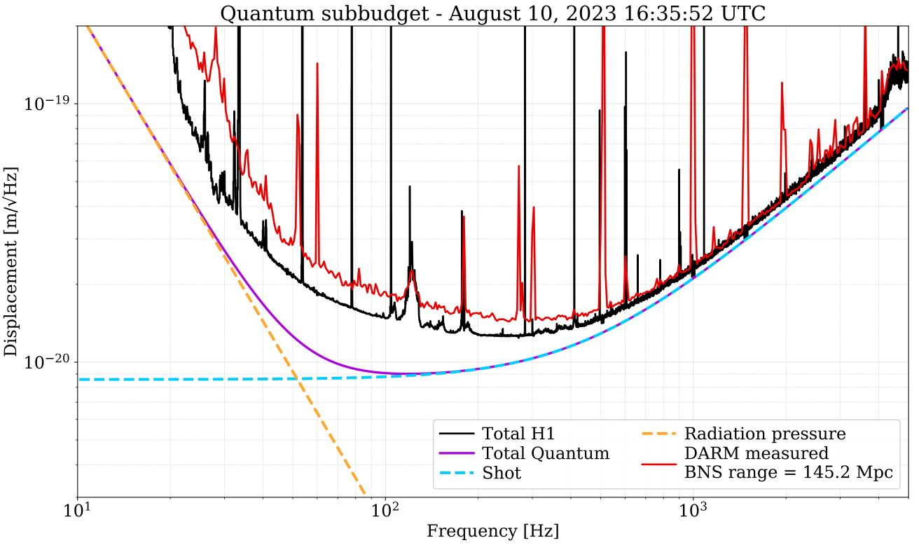
start = 1375720570 span = 600 s DARM channel H1:GDS-CALIB\_STRAIN\_CLEAN
