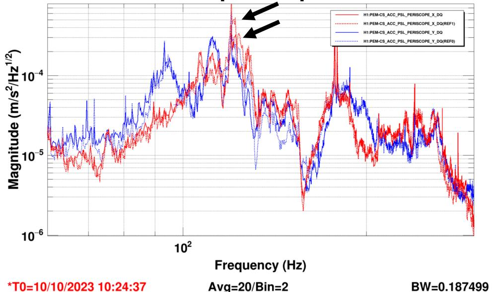
Solid lines: after periscope tuning and HVAC SF2 shutdown
