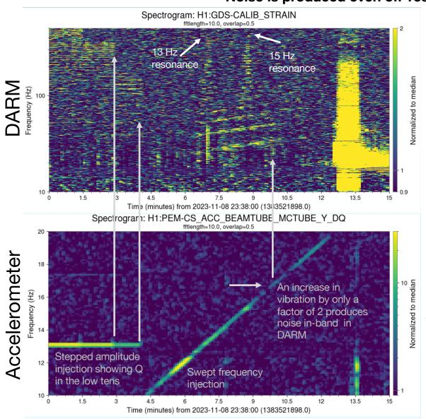
Below: An injection that is roughly consistent with the HVAC increase produces noise in DARM.
