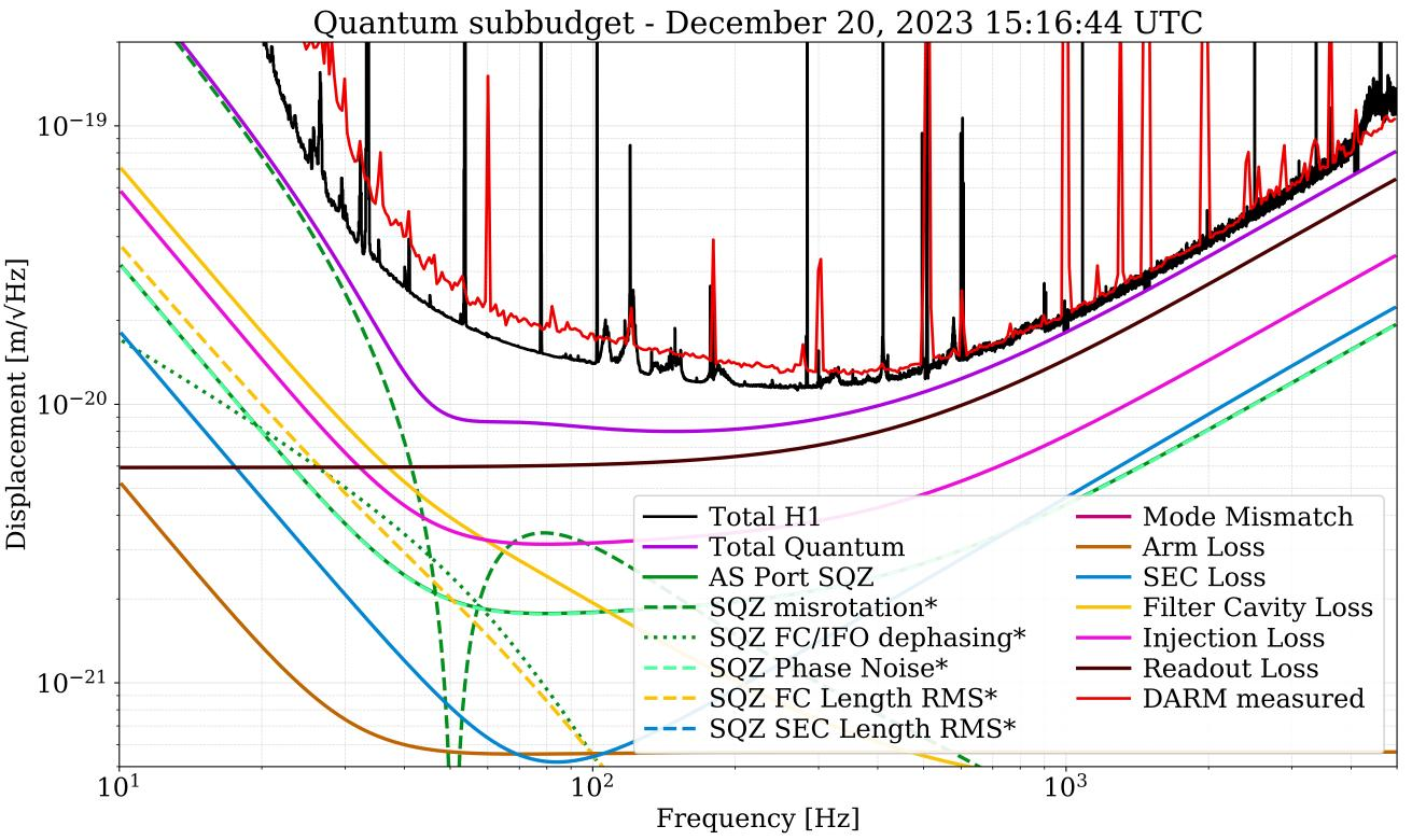
start = 1387120622 span = 600 s DARM channel H1:GDS-CALIB STRAIN CLEAN
