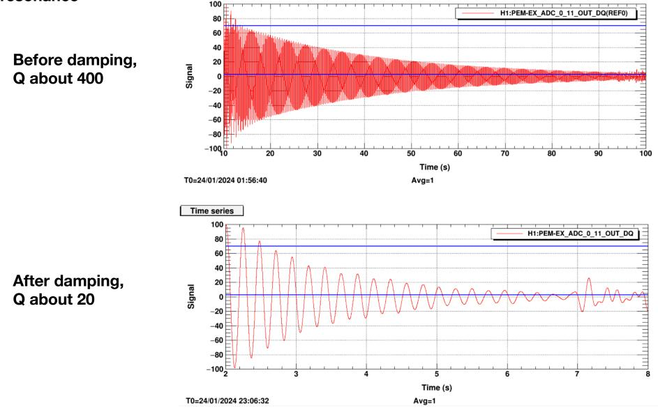
Laser vibrometer spectra before and after damping
