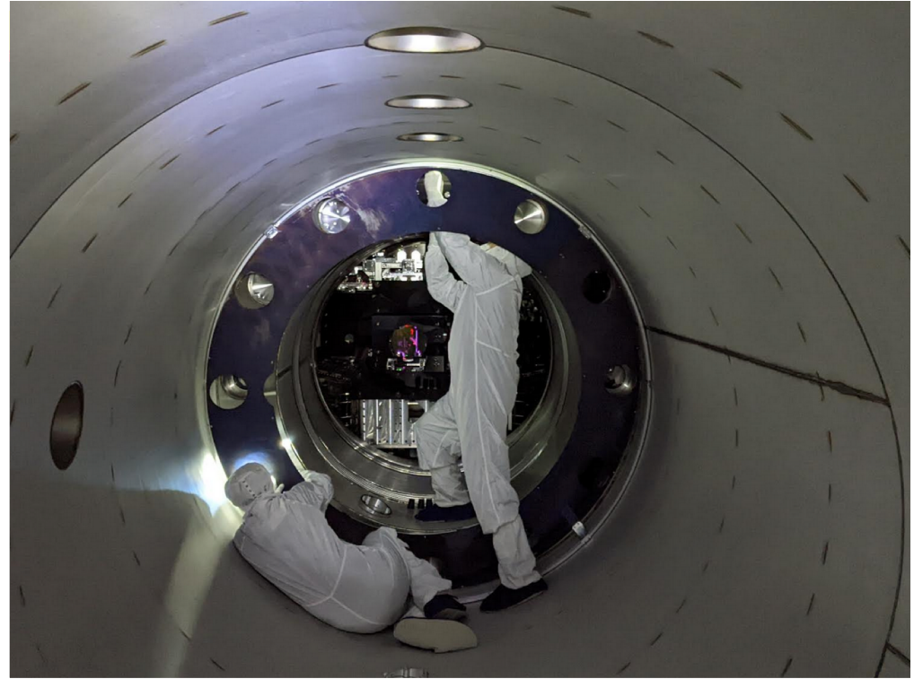
Tony and Corey installing nozzle baffles near HAM 2)
