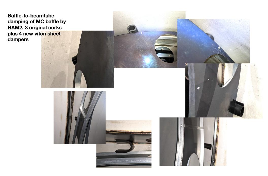
Examples of baffle panel damping. All panels were damped similarly. Most panels had been damped previously, so the increase was under a factor of two.
