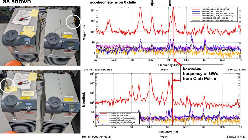
Peaks that are largest when accelerometer is on Y chiller
